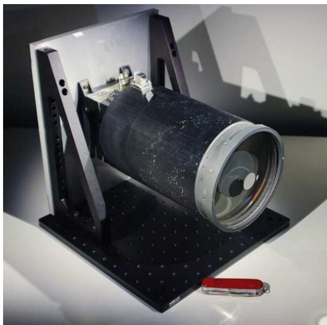
Figure 12. The MRO Context Camera (CTX) telescope and electronics on a support bracket. Swiss Army knife for scale. A Schmidt-type catadioptric optical design, which uses lenses to focus light on a primary mirror, is used to achieve a large field of view. The telescope tube is made of graphite/cyanate-ester composite material.
